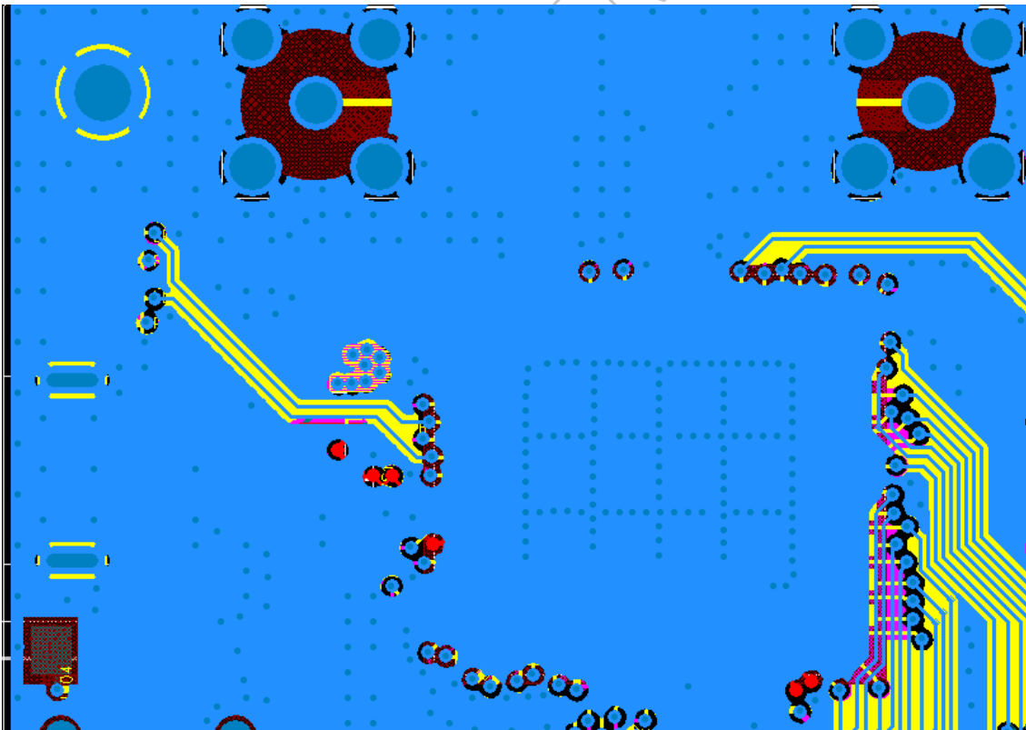
Figure 25: USB trace on layer 2
